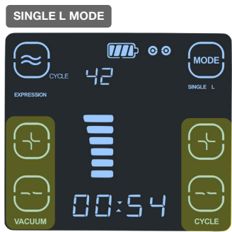
Increasing or decreasing the vacuum level and/or cycle will affect the currently selected side only.
