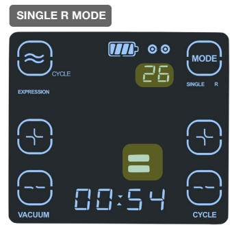
Screen will show the current vacuum level and cycle for the selected side.
